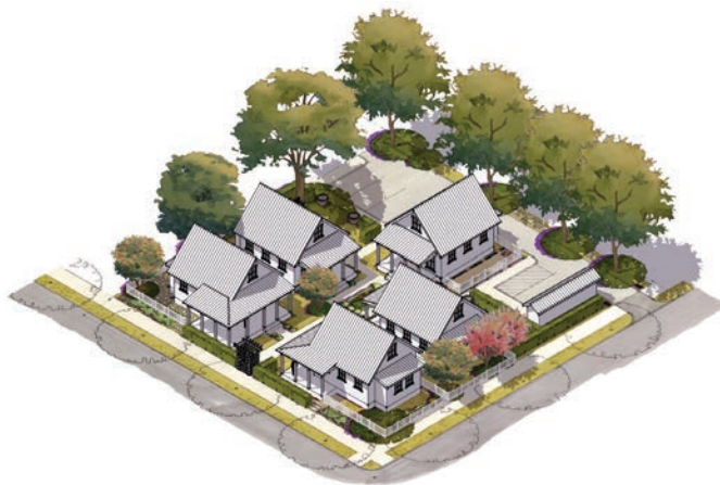
◀ In this site plan, five cottage-style homes (of about 650 square-feet each) fit on a 14,976-square-foot (or .34 acre) lot.
